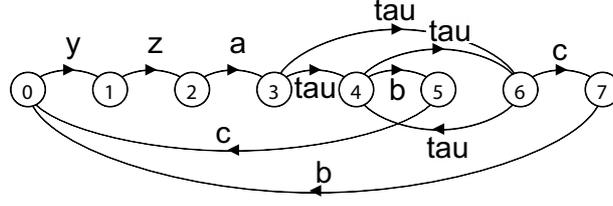
Figure 18: An implementation of the MTS in Figure 17
